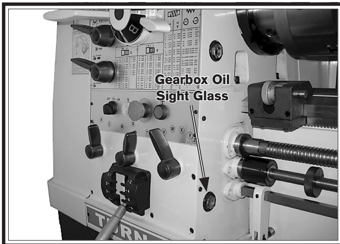
Figure 102. Location of quick-change gearbox oil sight glass.
